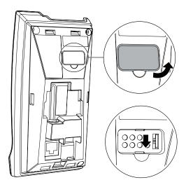
2. Tapping the handset power tact-switch to the off position. When the telephone base and handset successfully enters the energy-saving charging mode, all keys on the telephone base should not respond.
