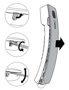
2. Unplug the battery connector from the socket and then remove the battery from the handset battery compartment.
