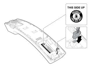
4. To replace the handset cover, align all the tabs on the handset cover against the corresponding grooves on the handset, then firmly push downward until all the tabs lock in the grooves. Then install the screw.
