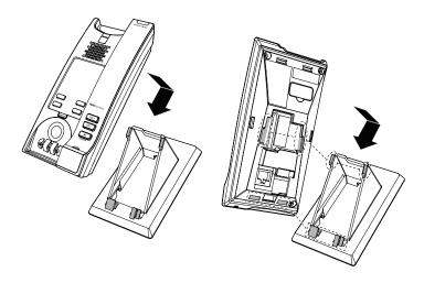
TO UNMOUNT THE BASE STAND Simply slide up and lift the telephone base from the base stand.
