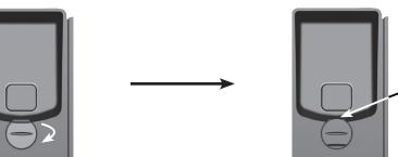
Unplug the telephone line cord from the telephone wall jack. Then press the large tab on the mounting bracket to remove it from the upper groove on the telephone base.
