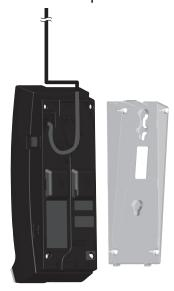
3. Install the telephone base as shown below. Then connect the coiled handset cord to the telephone base.
