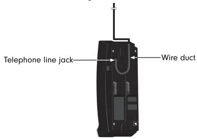
2. Position the mounting bracket as shown. Insert the two small tabs of the mounting bracket into the lower slots on the telephone base. Then press the large tab on the mounting bracket and firmly push it into the upper groove on the telephone base.
