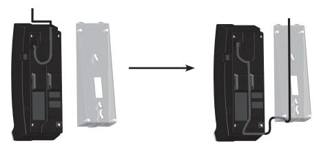
4. Mount the telephone base on the wall by aligning the eyelets with the mounting studs of the wall plate. Then slide the telephone base down on both mounting studs until it locks into place. Place the handset on the telephone base cradle.
