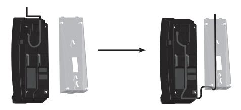
4. Mount the telephone base on the wall by aligning the eyelets with the mounting studs of the wall plate. Then slide the telephone base down on both mounting studs until it locks into place. Place the handset on the telephone base cradle.
