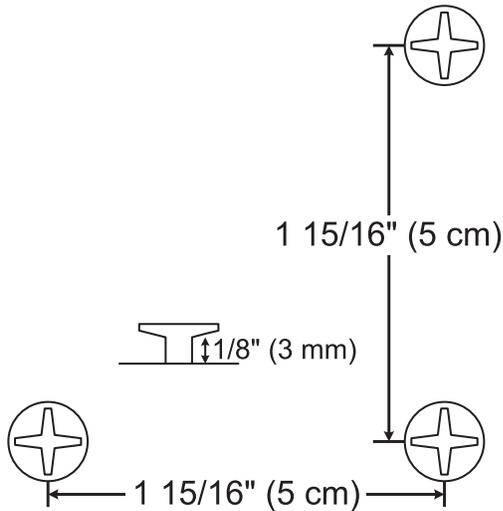
2. Tighten screws until only 3 mm (1/8 inch) of the screws are exposed.
