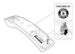
4. To replace the handset cover, align all the tabs on the handset cover against the corresponding grooves on the handset, then firmly push downward until all the tabs lock in the grooves. Then install the screw.
