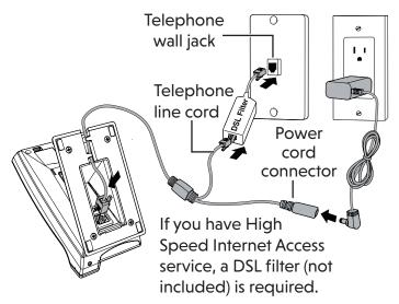
2. When the telephone base has been initially installed, make sure the power adapter is securely plugged into an outlet not controlled
