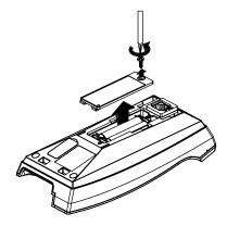
2. Remove the old batteries. If there is corrosion at the battery contacts, clean them with a cotton swab or a soft, lint-free cloth.
