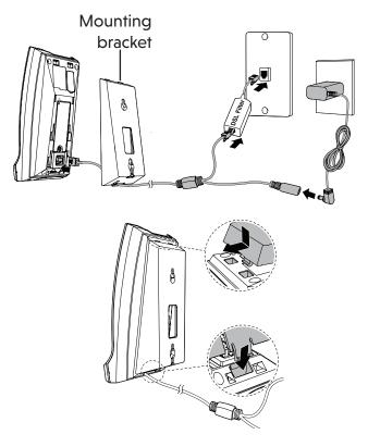
3. Mount the telephone base on the wall by positioning the eyelets on the telephone base and the mounting bracket against the mounting studs. Then slide the telephone base down on both mounting studs until it locks into place.
