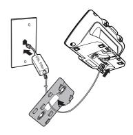
2. Align and place the wall mount bracket on the standard wall plate.
