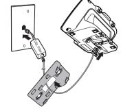
Align and place the wall mount bracket on the standard wall plate.
