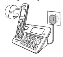
Once you have installed the battery, the handset LCD display indicates the battery status (see the table below).
