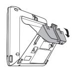
3. Plug the telephone line cord (or DSL filter) into the wall jack. Align the holes on the back of the telephone base with the standard wall plate. Slide the bracket down until it clicks securely in place. Connect the power adapter to the telephone base and an electrical outlet not controlled by a wall switch.
