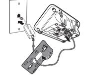
Align the holes on the bracket with the standard wall plate and slide the bracket down until it clicks securely in place.
