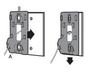
Align the grooves on the telephone base with the tabs on the wall mount bracket, and then slide it down until it clicks securely in place.
