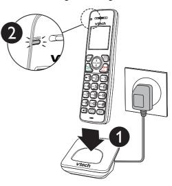
Once you have installed the battery, the handset LCD display indicates the battery status (see the table on next page).
