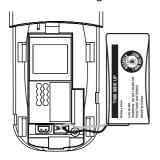
3. Slide the battery compartment cover towards the center of the handset until it clicks into place.
