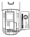
Place the battery with the label THIS SIDE UP facing up and the wires inside the battery compartment.
