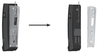
3. Turn the mounting bracket upside down. Remove the telephone line cord from the wire duct and then route it through the rectangular hole on the mounting bracket. Insert the small tabs on the mounting bracket into the upper slots on the telephone base. Then press the large tab on the mounting bracket and firmly push it into the lower groove on the telephone base.
