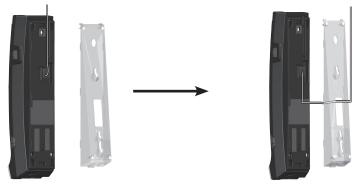
4. Mount the telephone base on the wall by aligning the eyelets with the mounting studs of the wall plate. Then slide the telephone base down on both mounting studs until it locks into place. Place the handset on the telephone base cradle.
