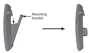
3. Mount the telephone base on the wall by aligning the eyelets with the mounting studs of the wall plate. Then slide the telephone base down on both mounting studs until it locks into place.
