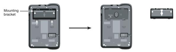
3. Rotate the mounting bracket. Insert the tabs of the mounting bracket into the middle grooves on the telephone base as shown below. Then press the tabs and push the mounting bracket into the lower grooves on the telephone base until they lock securely.
