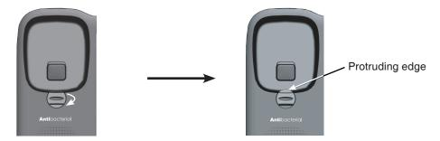
3. Turn the telephone base over with the bottom side facing up. To remove the mounting bracket, press the tabs of the mounting bracket in the direction indicated below to release and remove it from the telephone base.
