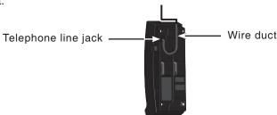
2. Position the mounting bracket as shown. Insert the two small tabs of the mounting bracket into the lower slots on the telephone base. Then press the large tab on the mounting bracket and firmly push it into the upper groove on the telephone base.
