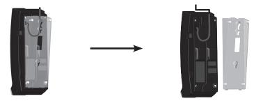
3. Turn the mounting bracket upside down. Remove the telephone line cord from the wire duct and then route it through the groove on the bottom part of the mounting bracket. Insert the small tabs on the mounting bracket into the upper slots on the telephone base. Then press the large tab on the mounting bracket and firmly push it into the lower groove on the telephone base.
