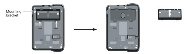
4. Rotate the mounting bracket. Insert the tabs of the mounting bracket into the middle grooves on the telephone base as shown below. Then press the tabs and push the mounting bracket into the lower grooves on the telephone base until they lock securely.
