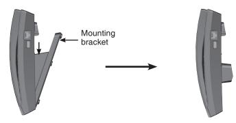
4. Plug the Cat-5 network cable back into the network wall jack with Power over Ethernet (PoE). Then slide the telephone base down on both mounting studs until it locks into place.
