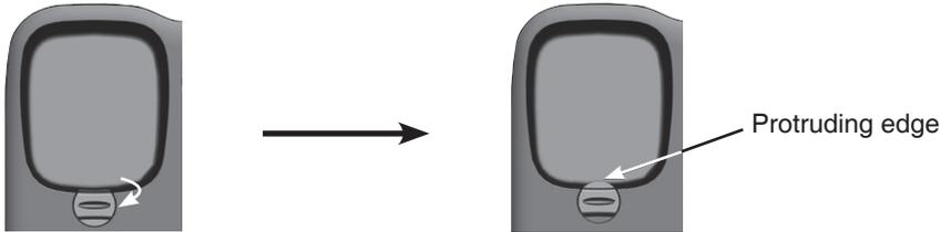
3. Turn the telephone base over with the bottom side facing up. Press the tabs of the mounting bracket as the direction indicated below to release and remove the mounting bracket from the telephone base.
