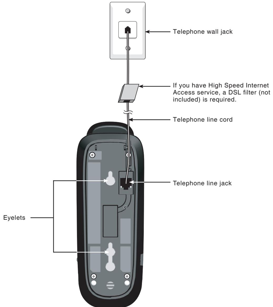
2. After installing the telephone base, mount it on the wall by positioning the eyelets on the telephone base against the mounting studs of the wall plate. Then slide the telephone base down on both mounting studs until it locks into place.
