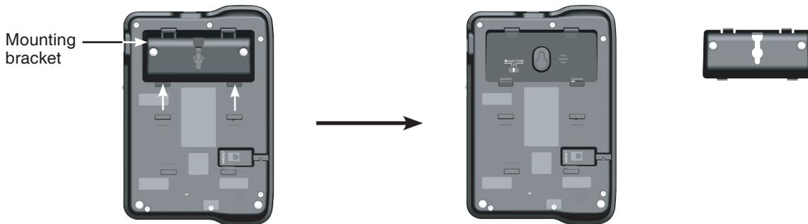
3. Rotate the mounting bracket. Insert the tabs of the mounting bracket into the middle grooves on the telephone base as shown below. Then press the tabs and push the mounting bracket into the lower grooves on the telephone base until they lock securely.
