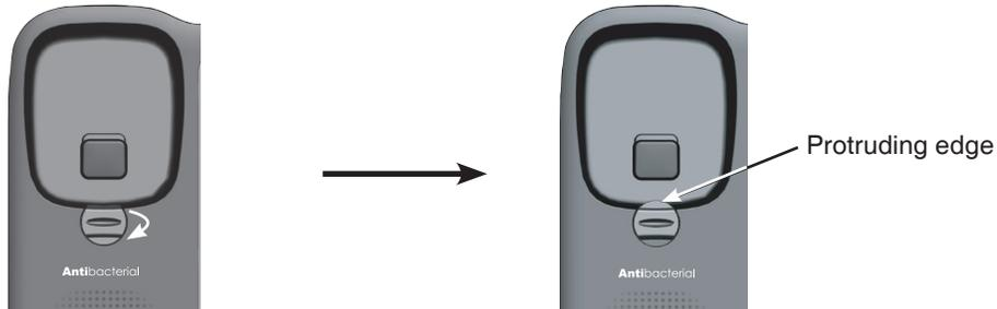
2. Turn the telephone base over with the bottom side facing up. Press the tabs of the mounting bracket as the direction indicated below to release and remove the mounting bracket from the telephone base.
