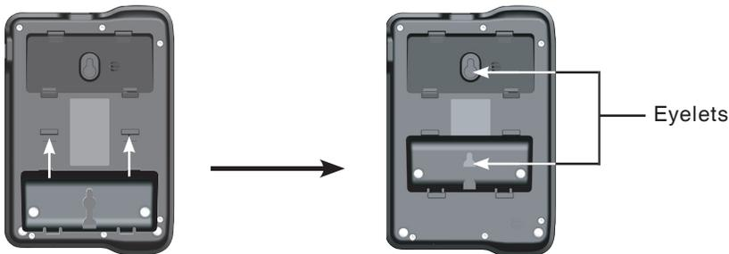
5. Mount the telephone base on the wall by positioning the eyelets on the telephone base and mounting bracket against the mounting studs of the wall plate. Then slide the telephone base down on both mounting studs until it locks into place.
