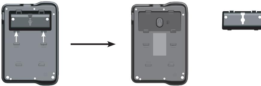
4. Rotate the mounting bracket. Insert the tabs of the mounting bracket into the middle grooves on the telephone base as shown below. Then press the tabs and push the mounting bracket into the lower grooves on the telephone base until they lock securely.
