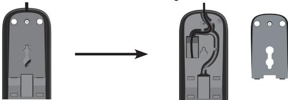
4. Rotate the mounting bracket. Insert the tabs of the mounting bracket into the lower grooves of the charging base. Then tighten the screw to affix the mounting bracket.
