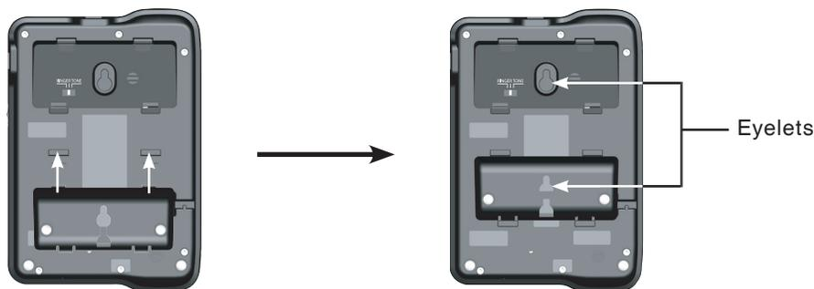
4. Mount the telephone base on the wall by positioning the eyelets on the telephone base and the mounting bracket against the mounting studs. Then slide the telephone base down on both mounting studs until it locks into place.
