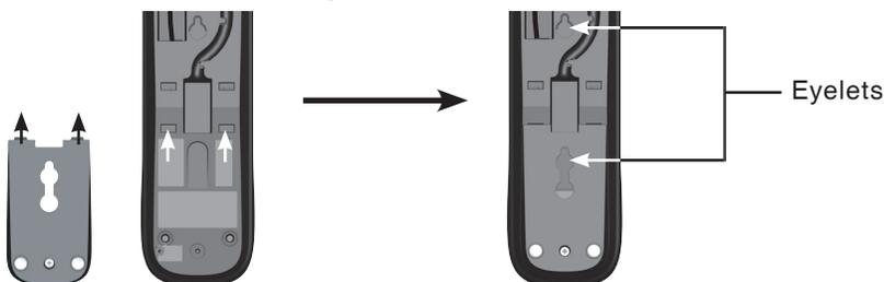
5. Mount the charging base on the wall by positioning the eyelets on the charging base and the mounting bracket against the mounting studs of the wall plate. Then slide the charging base down on both mounting studs until it locks into place.
