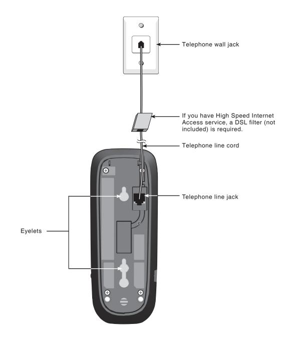
2. After installing the telephone base, mount it on the wall by positioning the eyelets on the telephone base against the mounting studs of the wall plate. Then slide the telephone base down on both mounting studs until it locks into place.
