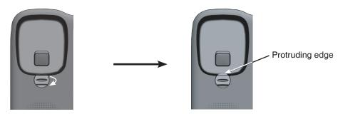
2. Turn the telephone base over with the bottom side facing up. Press the tabs of the mounting bracket as the direction indicated below to release and remove the mounting bracket from the telephone base.
