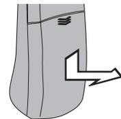
1. Remove the battery case by pressing on the ridged lines and sliding downward.
