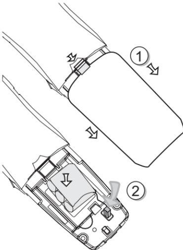
1. Remove the battery cover by pressing on the indent and sliding downward.
