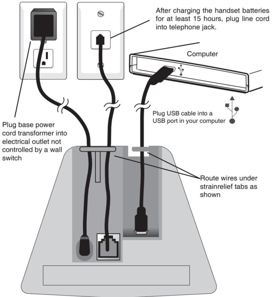
Underside of telephone base
