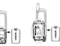
3. Align the cover flat against the battery compartment, then slide it upwards until it clicks into place.
