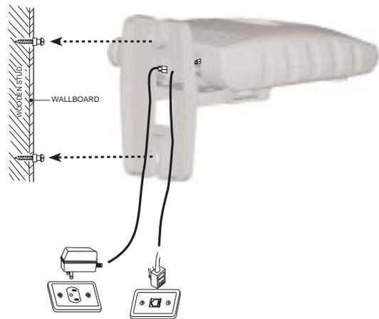
1. **Choose a spot near an electrical outlet and a telephone jack.** Your phone requires a modular telephone jack and a standard electrical outlet (120V AC). The power cord is six feet long; make sure there is an electrical outlet within reach of the base. The outlet should not be controlled by a wall switch. If the switch is ever turned off, the phone will not operate.
