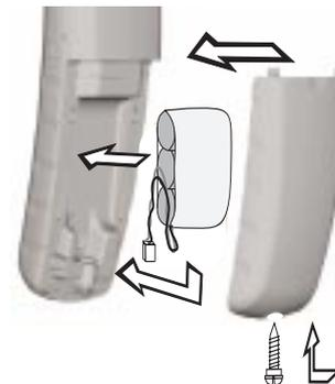
1. Remove the locking screw on the bottom of the Handset, then slide the battery cover off by gently pressing on the recessed area with a downward motion.
