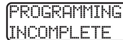
Unsuccessful programming can result from not correctly completing the programming sequence. For example, if after entering a number on the LCD and entering program mode, the **OFF** key were pressed instead of entering a valid memory location, the "PROGRAMMING INCOMPLETE" message would appear. If this message appears, simply repeat the programming sequence.
