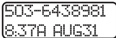
Pressing the **(◀\*)** key displays the next lower in sequence call record. Likewise, pressing the **(▶#)** key displays the next higher in sequence call record. The higher the call number, the older the call.
