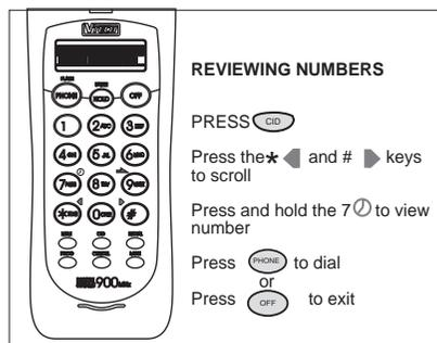
To find out the corresponding phone number as well as the date and time of the call, press and hold the **7 (🕒)** key. The date and time will be shown. Releasing the key will again show the caller's name.
