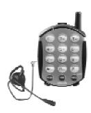
Make sure you have a compatible 2.5mm Headset with you. Locate the Headset Jack on the Belt Pack of your **VT1411**. Connect the plug on the Headset to the jack on the cordless Belt Pack. The plug should fit securely. Do not force the connection. See illustration.
