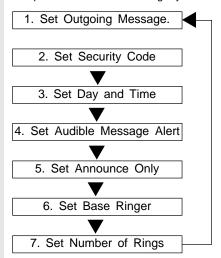
During Answering System setup, the display will flash " -- ". If no key is pressed for 20 seconds, the Answering System will beep, and exit program mode. You can also exit program mode at any time by pressing any **MAILBOX** key.
