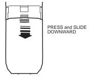
2. Slide the Handset battery cover down, and remove it from the Handset.
