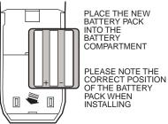
Install the BATTERY PACK, with the metal contacts facing down and aligned with the Handset contacts. Replace Handset battery cover.
