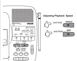
During playback, you can change the playback speed by simply holding down ◄ (SLOW) or ►► (QUICK) to the desired speed during playback. There are 3 playback speeds (SLOW/NORMAL/QUICK). The default speed is normal. Playback speed will return to normal once you exit the playback mode.
